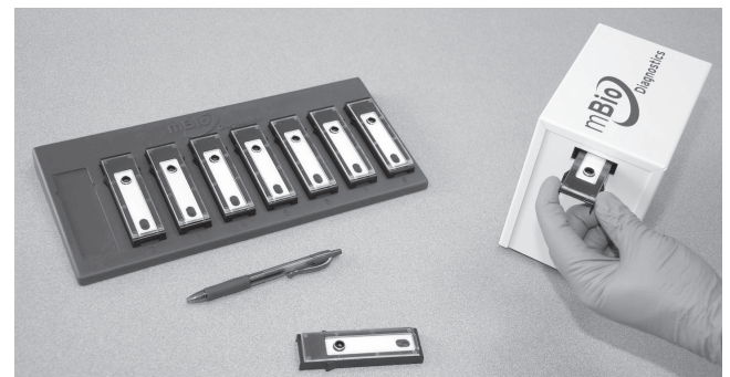
FIG. 1. (Top) Schematic representation of the multiplexed fluorescence immunoassay and disposable assay cartridge. A protein microarray is printed to a plastic planar waveguide which is bonded to a plastic upper component to define a flow channel. Sample, wash, and detect reagents are introduced via a fluid inlet. Illumination of the assay surface is via the evanescent field generated down the length of the multimode waveguide. The array is imaged in a single field of view through the plane of the waveguide. (Bottom) MBio instrument and rack of assay cartridges.
