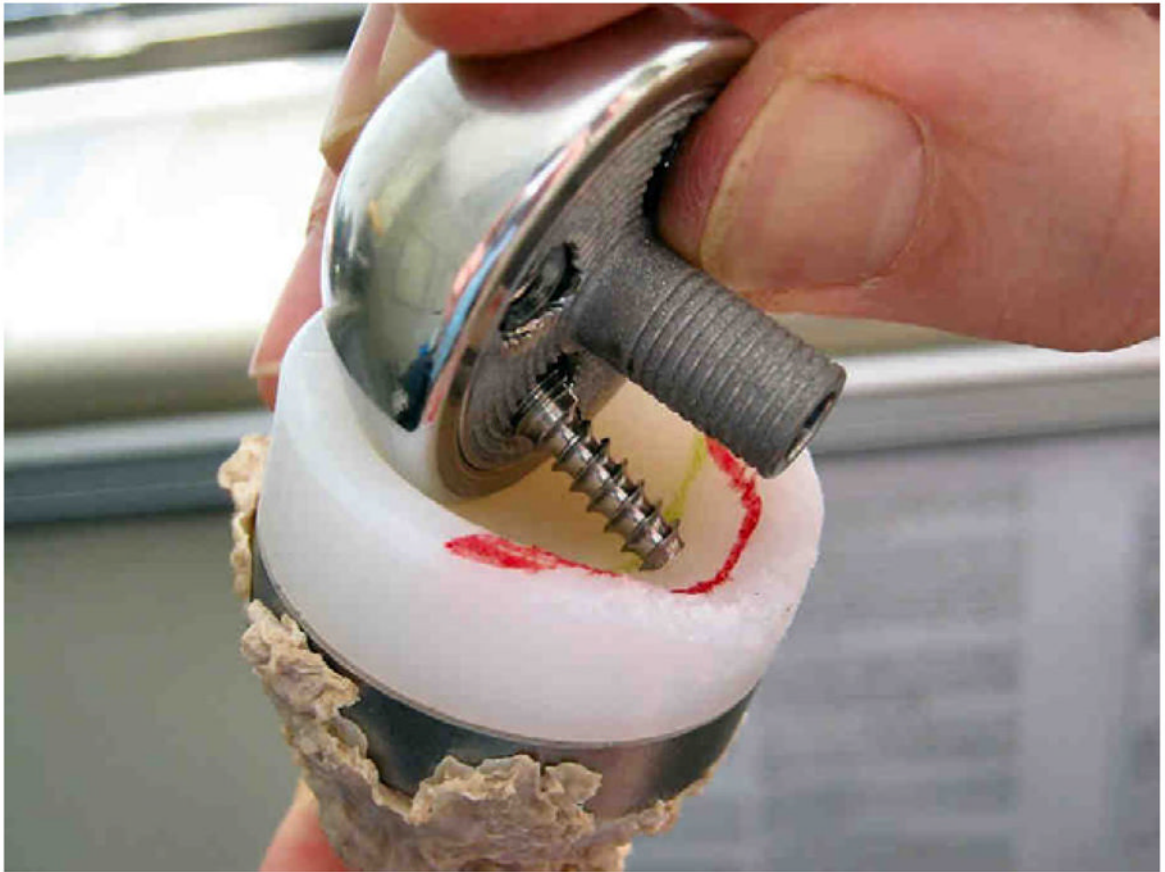
Figure 4. Retrieved reverse total shoulder implant that was implanted for 3.3 years with evidence of wear on the rim from the screw as well as abrasive wear on the intended bearing surface from the broken screw.
