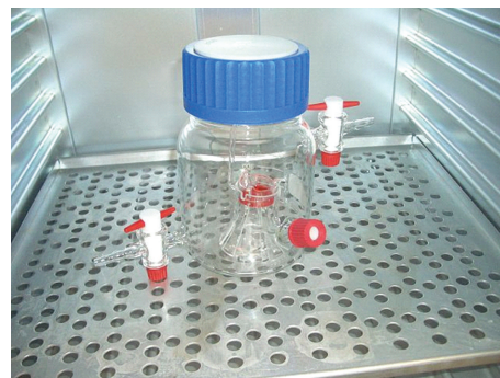
FIGURE 1: Modified glass flask for exposure of cells to volatile metal(loid) species. Cells were grown on permeable membranes. Exposure occurred through the membrane.
