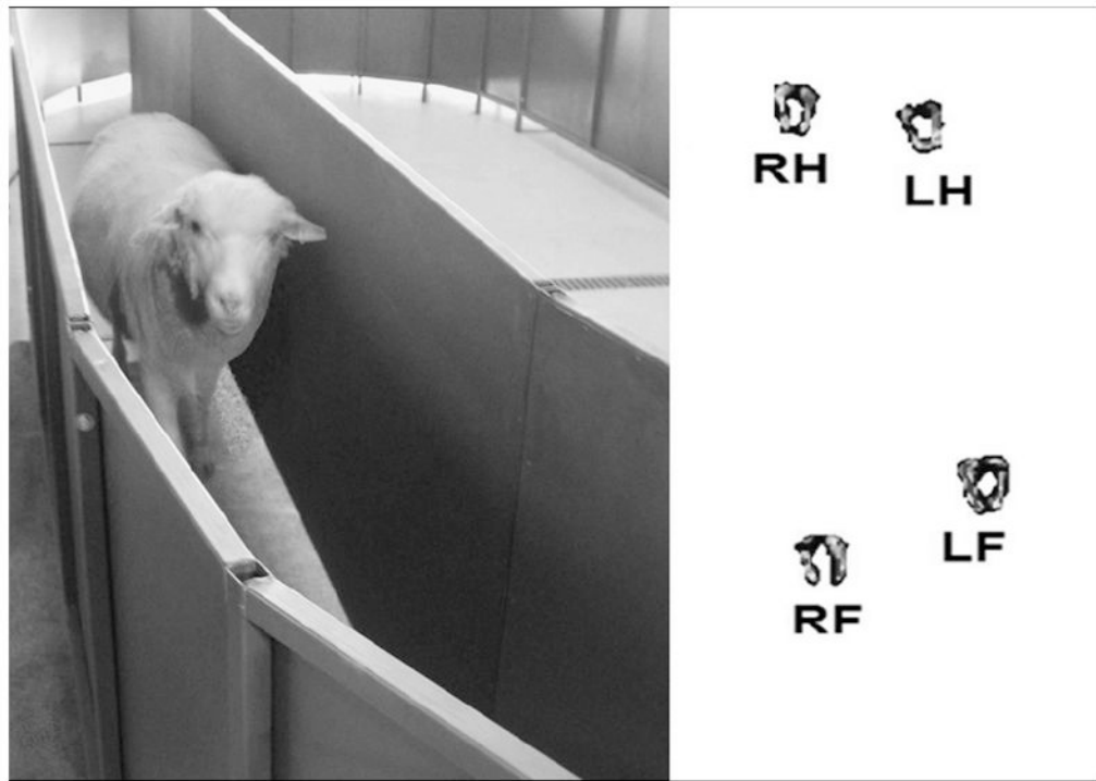
Figure 2. (Left) Photograph of a sheep standing on the pressure mat within the enclosure. (Right) Output of the pressure sensing mat showing the Right Hindlimb (RH), Left Hindlimb (LH), Right Forelimb (RF), and Left Forelimb (LF).
