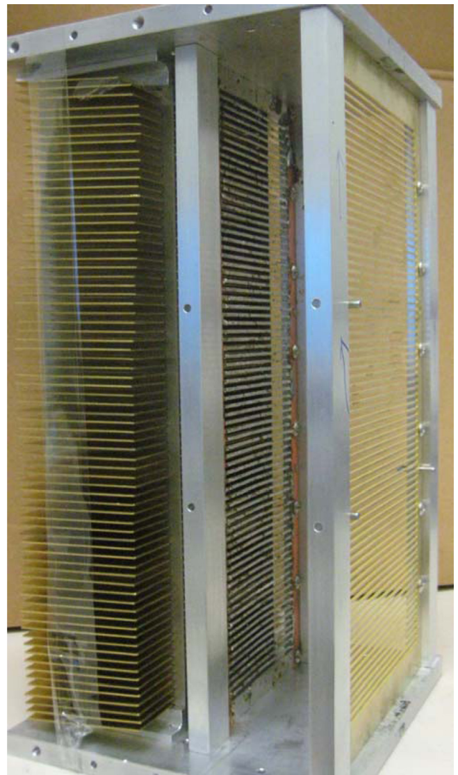
FIG. 4. Multislit collimator of the TBCT benchtop. It comprises a stack of brass plates aligned at different angles and two plates with 75 precisely machined slot openings.
