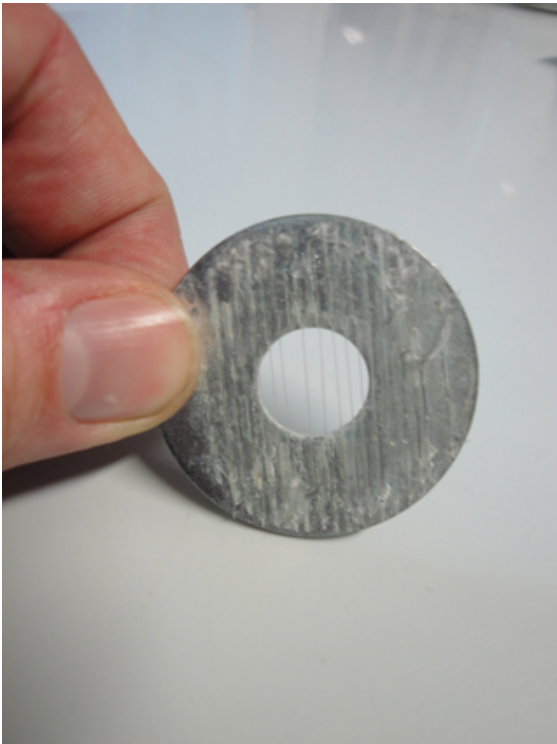
Supplemental figure 3. Lung lobe fixation. After preparation of the right lung lobe the organ is fixed in a Petri dish by use of a laboratory-made flat washer that is covered by a set of parallel nylon threads.
