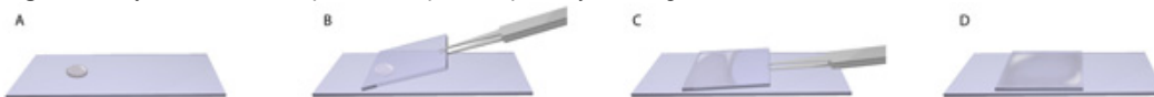
Figure 3. Mount the coverslips with the cell side down on clean glass microscope slides using Mowiol mounting reagent.
