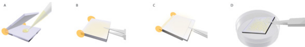
Figure 1. Coat 22 X 22 mm glass coverslips with poly D lysine and place one coated side up in each 35 mm dish.
