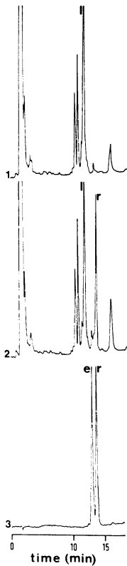
Figure 6: HPLC profile of recombinant and authentic eglin c (absorbance unit full scale, 220 nm: 0.2). 50 \mu l bacterial lysates were mixed with 50 \mu l 0.18 M acetic acid, centrifuged and the supernatants injected.
