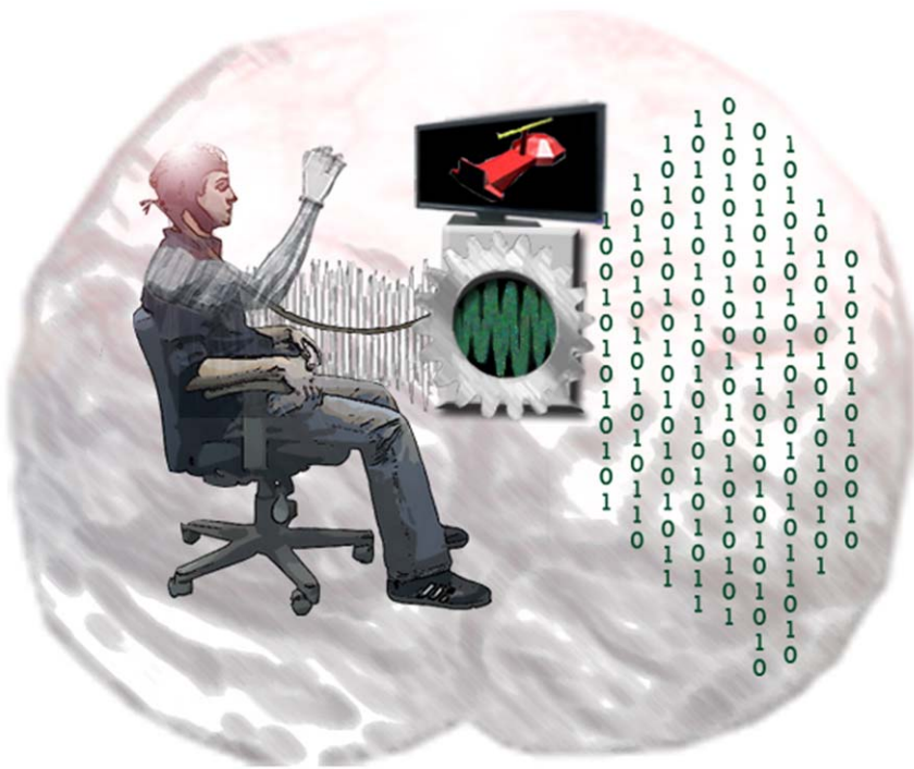
Figure 1. A diagrammatic representation of the presented BCI system. Using specifically trained motor imaginations learned in single dimensional cursor tasks, subjects control the three-dimensional movement of a virtual helicopter. Raw EEG is temporally and spatially filtered to produce individualized control signal components. These components are weighted and digitized in a subject specific manner and output to influence control in the virtual world. doi:10.1371/journal.pone.0026322.g001
