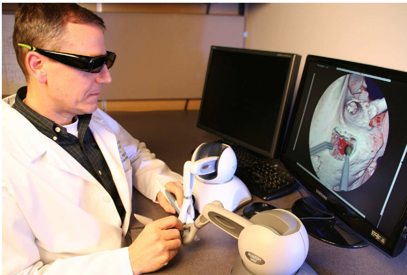
Figure 1. User in current temporal bone simulator from The Ohio State University. Interface includes stereo visual and dual haptic feedback devices for procedural interaction.
