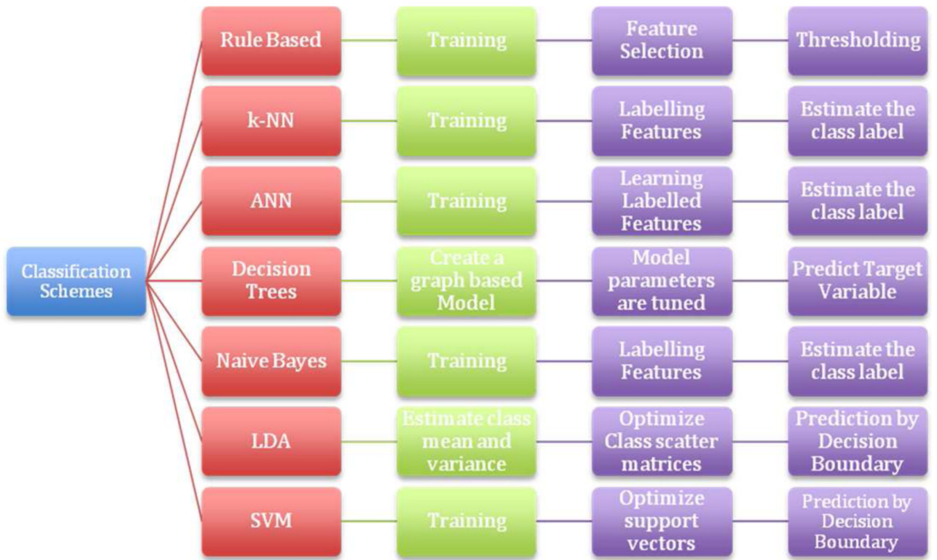
Figure 6. The most commonly used classifiers for CAD systems, with their organizational principles.
