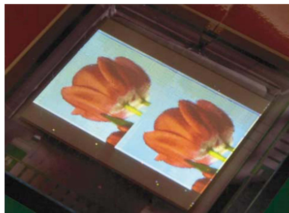
Figure 10 Image of an organic display panel developed by Philips Electronics. Reproduced from [75]. Copyright Nature Publishing Group, 2004.
