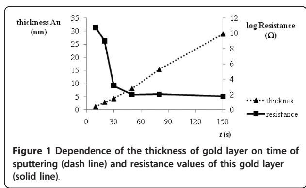
**Figure 1** Dependence of the thickness of gold layer on time of sputtering (dash line) and resistance values of this gold layer (solid line).
