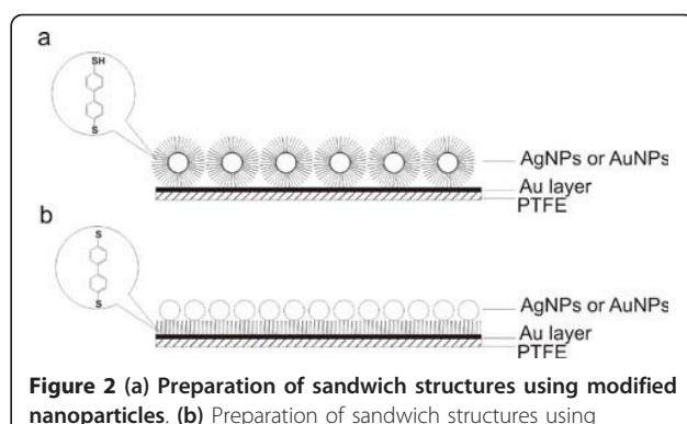
**Figure 2** (a) Preparation of sandwich structures using modified nanoparticles. (b) Preparation of sandwich structures using modified gold layer.
