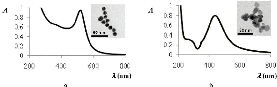
**Figure 3** (a) UV-Vis absorption spectra of the AuNPs and TEM image (in excision); (b) UV-Vis absorption spectra of the AgNPs and TEM image (in excision).
