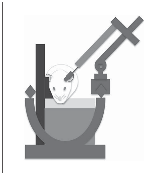
Fig. 1. RTBI model. Anesthetized animal is placed against a wooden L-shaped frame secured within a student stereotaxic frame.
