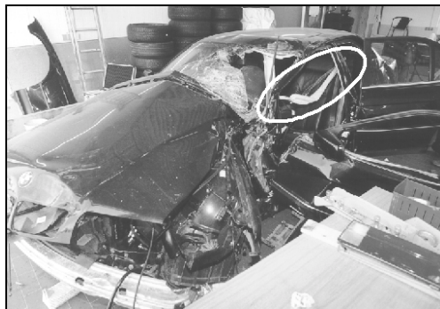
Fig. 16 – Damage to the BMW 730d
