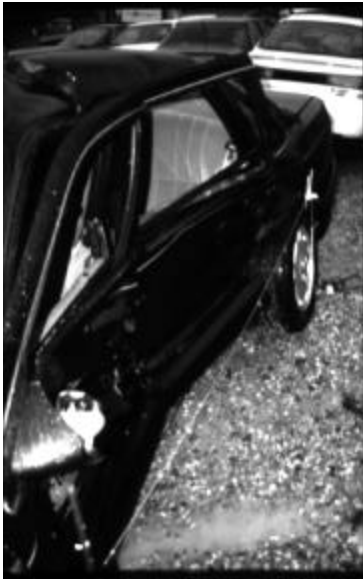
Figure 18. Damage to 1994 Ford Taurus in case GMP-004. CDC: 10-LPEW-3, maximum crush: 50 cm.
