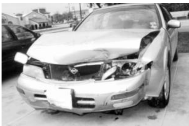
Figure 5. Damage to 1996 Nissan Maxima in case GMP-023. CDC: 12-FDEW-2; maximum crush: 32 cm.
