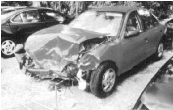
Figure 8. Damage to 1998 Chevrolet Cavalier in case GMP-026. CDC: 12-FDEW-3; maximum crush: 57 cm.
