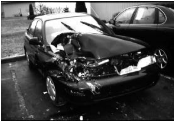
Figure 10. Damage to 1996 Toyota Corolla in case GMP-005. CDC: 12-FREW-1; maximum crush: 21 cm.
