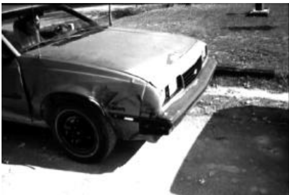
Figure 19. Damage to 1986 Chevrolet Cavalier in case GMP-001. CDC: 03-RFEW-2; maximum crush: 10 cm.
