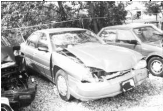
Figure 13. Damage to 1996 Chevrolet Lumina in case GMP-009. CDC: 12-FDEW-1; maximum crush: 14 cm.
