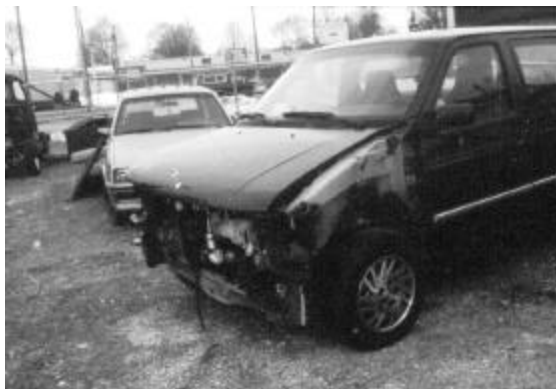
Figure 12. Damage to the 1993 Dodge Caravan in case GMP-006, with some parts removed. CDC: 01-FDEW-1; maximum crush: minor.
