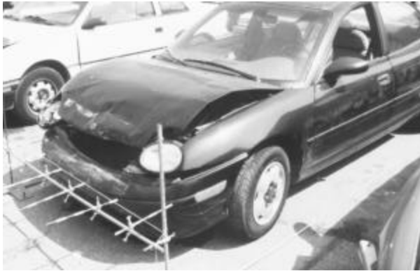
Figure 16. Damage to 1995 Dodge Neon in case GMP-027. CDC: 12-FDEW-1; maximum crush: 7 cm.
