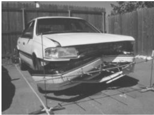
Figure 15. Damage to 1990 Ford Tempo in case GMP-022. CDC: 11-FYEW-2; maximum crush: 39 cm.
