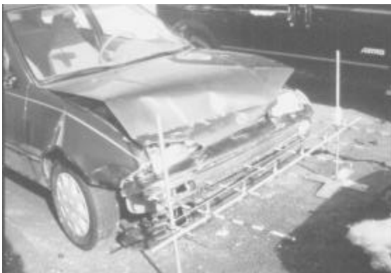
Figure 14. Damage to 1994 Suzuki Swift in case GMP-016. CDC: 01-FDEW-1; maximum crush: 19 cm.
