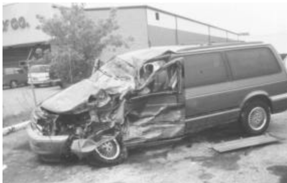
Figure 20. Damage to 1992 Plymouth Grand Voyager in case GMP-011. CDC: 10-LYAW-3; maximum crush: 23 cm.
