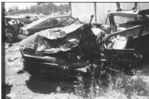
Figure 4. Damage to 1992 Saturn SL2 in case GMP-010, with roof removed by emergency personnel. CDC: 12-FYEW-5; maximum crush: 125 cm.
