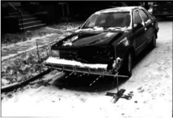
Figure 9. Damage to 1986 Ford Tempo in case GMP-003. CDC: 12-FYEW-1; maximum crush: 6 cm.
