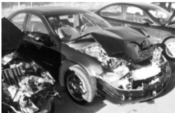
Figure 7. Damage to 1998 Dodge Stratus in case GMP-025. CDC: 12-FDEW-2; maximum crush: 40 cm.
