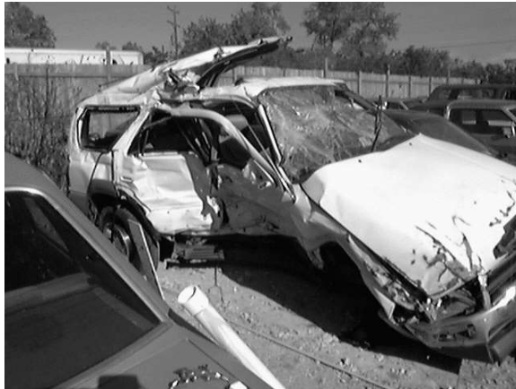
Figure 5. Fatal Injury in Rollover with Side Impacts but No Vertical Roof Deformation
