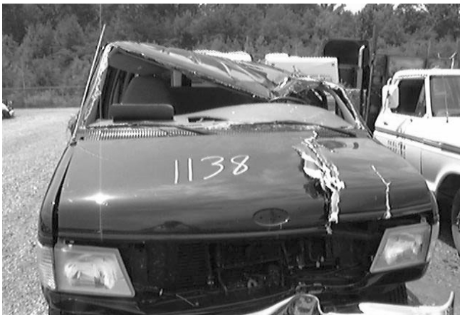
Figure 7. Minor Injury in a Rollover with Severe Roof Deformation
