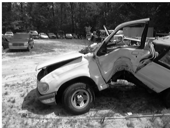
Figure 2. Arrested Roll: Results of Impact with Tree
