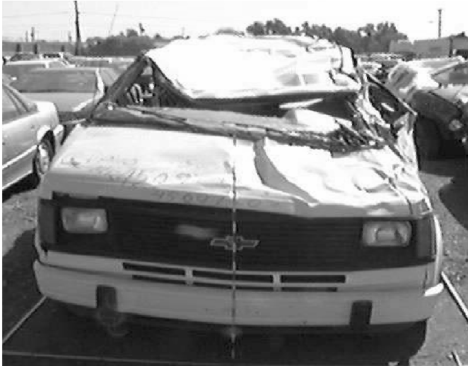
Figure 8. Another Example of Minor Injury in a Rollover with Severe Roof Deformation
