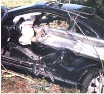
Case 470964. Driver lost control and drove into end of guardrail. Guardrail entered vehicle through right-front passenger window and eviscerated driver.
