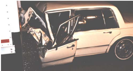
Case 170843. Driver ran into rear of large commercial truck. Severe under-ride resulted in stiff metal rear structure of truck striking head/face of driver. Massive intrusion (steering wheel in contact with driver's seatback).
