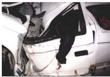
Case 171158. Vehicle went roof-first into tree. Impact at location of driver's head. Massive intrusion at driver's position and extensive head/neck injuries noted at autopsy.
