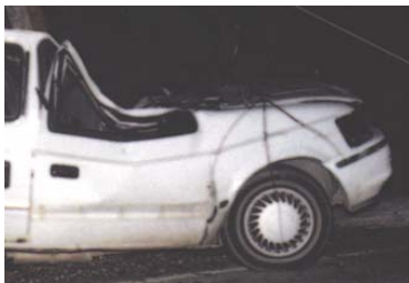
Case 171158. Vehicle went roof-first into tree. Impact at location of driver's head. Massive intrusion at driver's position and extensive head/neck injuries noted at autopsy.
