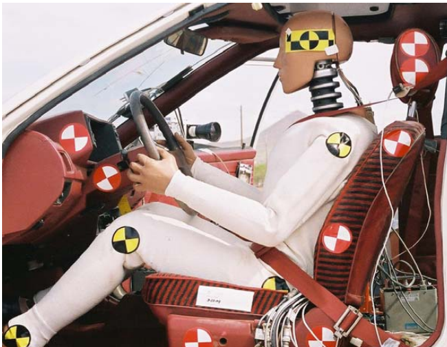
Figure 1 Photograph illustrating pre-impact positioning of ATD in vehicle-to-vehicle tests.
