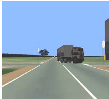
Fig 2: Highway hazard 4 - One truck is parked on shoulder of the right lane, a second truck in oncoming traffic turns left, encroaching on the participant's lane;
