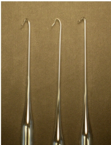
Figure 3. Three representative examples of glass hooks used to collect the viral DNA ghosts.
