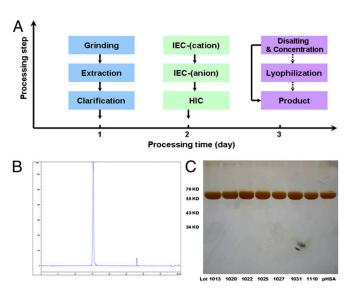
**Fig. 5.** Production of OsrHSA from transgenic rice seeds. (*A*) Large-scale process flow diagram of the purification of OsrHSA from transgenic rice seeds. (*B*) Purity analysis with reverse-phase HPLC (C<sub>4</sub>). (C) SDS/PAGE (silver staining) characterization of purified OsrHSA from large-scale production of lot nos. 1013 (99.09%), 1020 (99.42%), 1022 (99.60%), 1025 (99.45%), 1027 (99.59%), 1031 (99.55%), and 110 (99.09%). Purity was calculated by size-exclusion HPLC.
