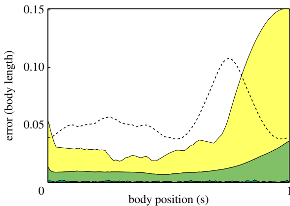
Figure 7. Error for midline fit. The midline was manually selected on a random set of 100 top-view frames. The distance was computed between the projected estimate and the manually generated midline was measured in the top camera frame. Dark green, minimum; light green, mean; yellow, maximum. For comparison with previous work, we also computed the mean error (dashed line) for a fish shape modelled as a bent ellipsoid [21]. (Online version in colour.)
