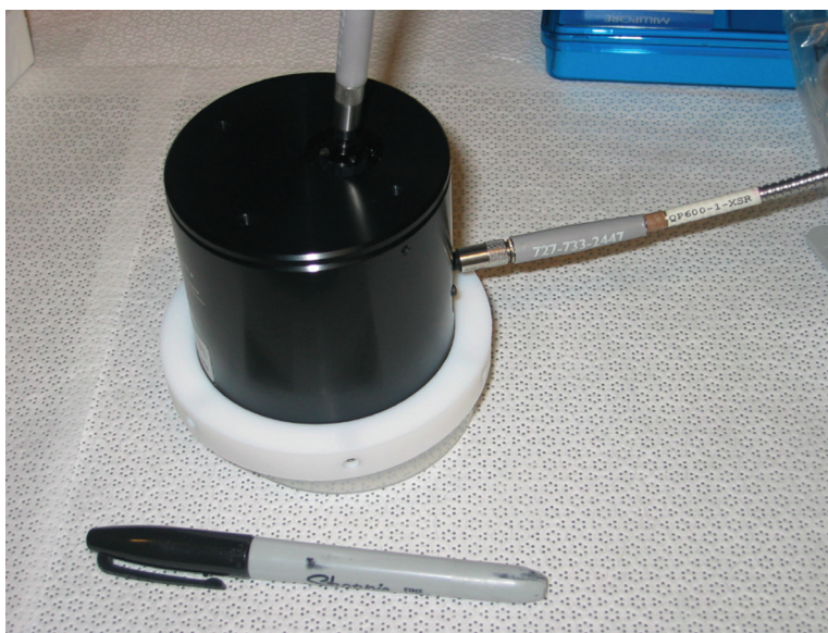
Figure 1. The modified integrating sphere showing the fiber optical cables with light in at 8^\circ off perpendicular and detector cable at 90^\circ . A reflective white layer of \text{BaSO}_4 was painted onto the bottom flat surface of the integrating sphere to minimize the loss of light interactive with the black enamel. To avoid flaking of this paint over time, a thin translucent layer of white Teflon (1.5 mm) was added to the bottom of the sphere (with a port to allow light in and out).
