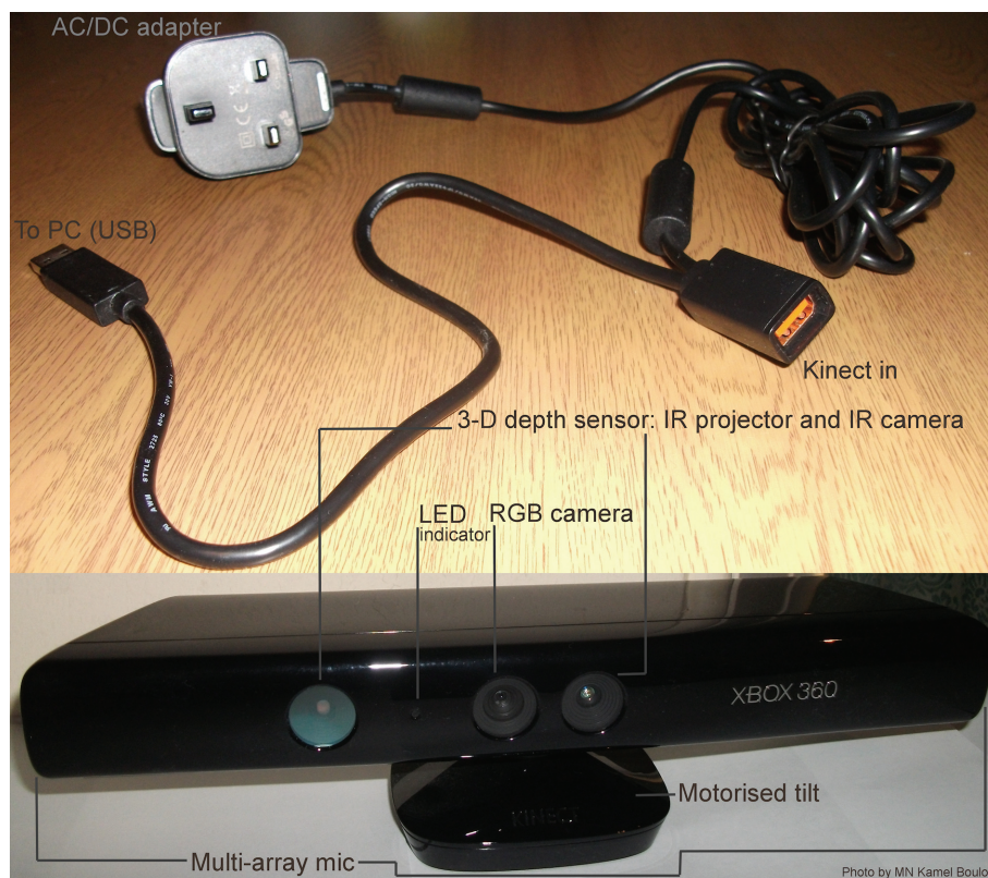
Figure 1 Anatomy of Microsoft Kinect.
