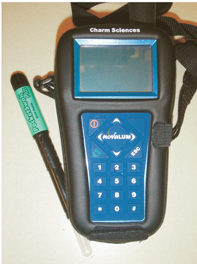
Figure 2. Luminometer (NovaLum, Charm Sciences) with dry swab (PocketSwab, Charm Sciences).
