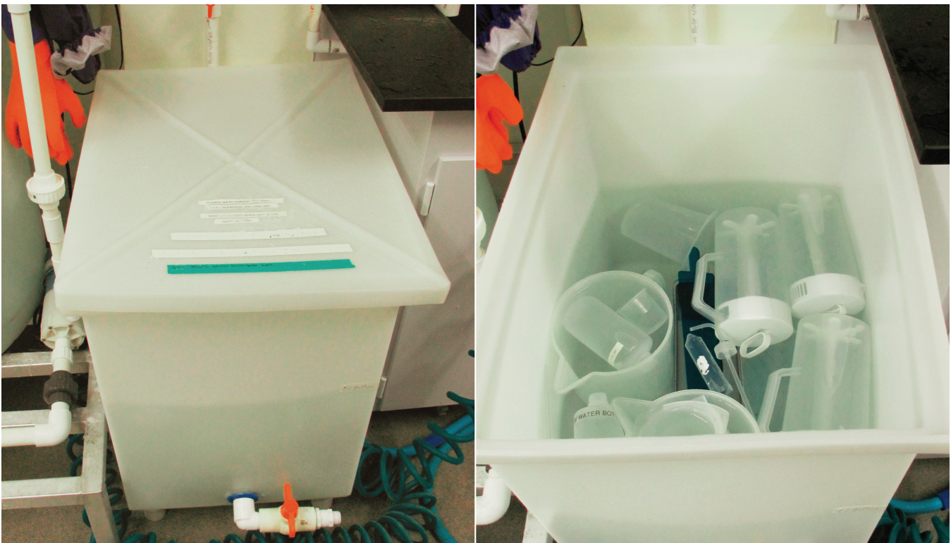
Figure 3. Opaque bins used to hold the 1.98% bleach disinfection solution. The lid was kept on the bin when not in active use, to decrease light exposure and minimize evaporation.
