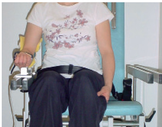
The Metitur Good Strength device for measurement of elbow flexion strength.
