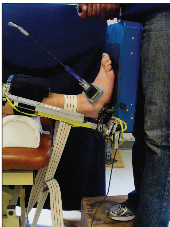
Figure 5. Anterior drawer testing and inversion testing as performed with the Hollis ankle arthrometer. Subject is supine with the foot/ankle secured in the device and strapped down to the table frame.
