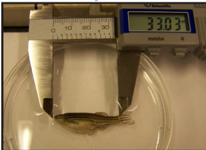
Figure 1. Measure the fish from snout to caudal peduncle using a digital mm caliper.
