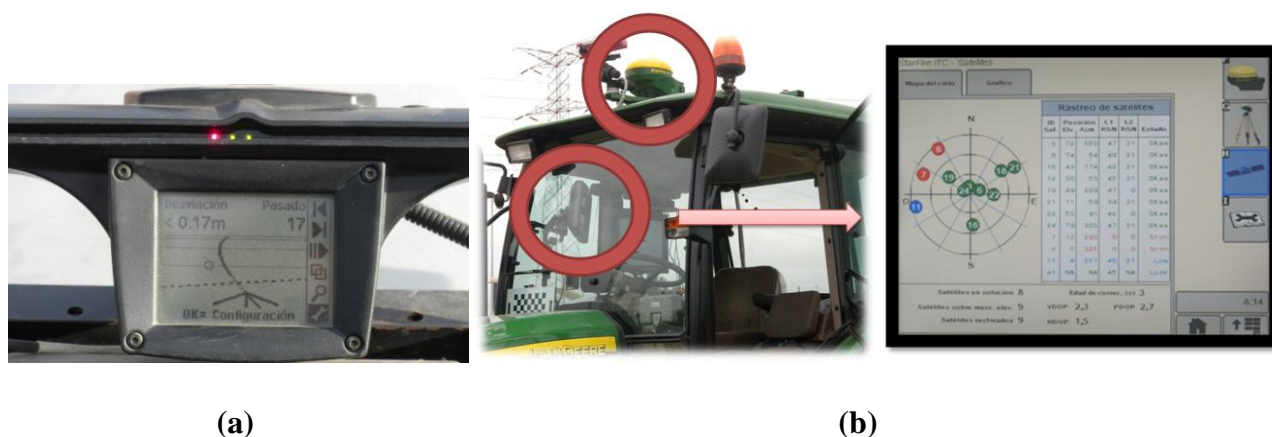
Figure 7. GPS for agricultural operations: (a) Lightbar steering assistance system. (b) DGPS onboard system.
