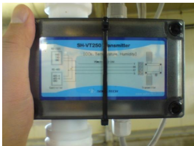
Figure 11. Wired Integrated Sensors.
