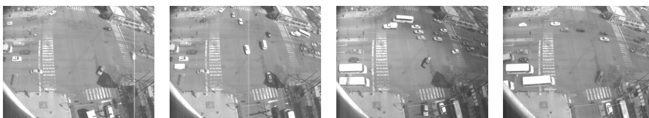
Figure 13. Sample of different environmental conditions at scene. The first two images represent situations where there are reflections caused by cars; the next two images represent rainy weather situations where the cloud sun occlusion causes changes in luminance conditions.
