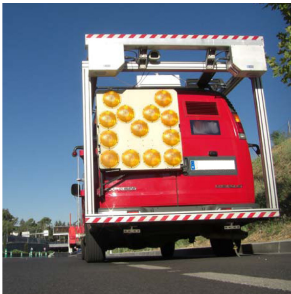
Figure 1. Rear of the vehicle used to acquire and store the road images.
