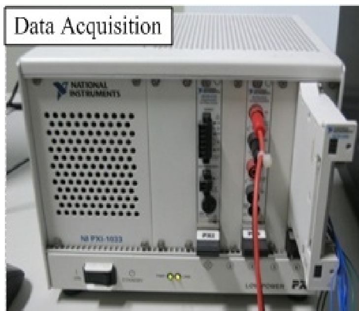
Figure 5. Resistance signal is picked up by Data Acquisition.
