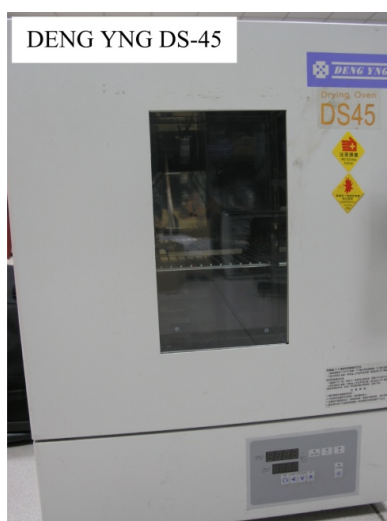
Figure 4. Calibration of micro temperature sensors in a thermal chamber.
