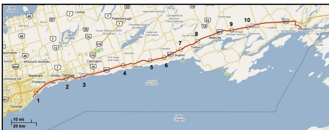
Figure 11. Road test trajectory from Toronto to Kingston. Circles indicate the locations of GPS outages.
