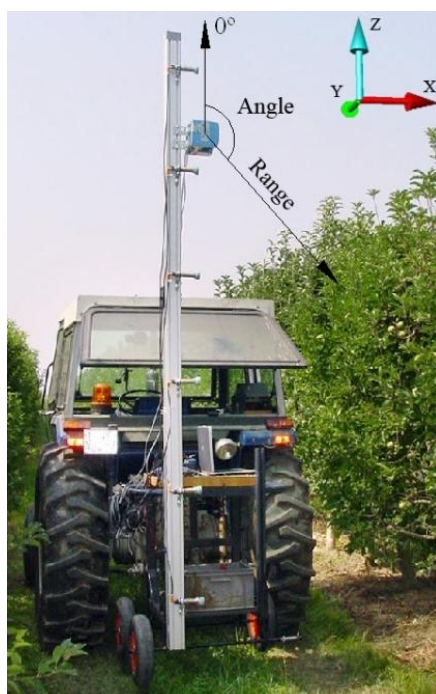
Figure 3. The impact points of the laser beam are determined in polar coordinates. The direction of the laser beam with an angle of 0^\circ is vertical and upward pointing. The Cartesian coordinate system (X,Y,Z) used in the field and laboratory is also shown.
