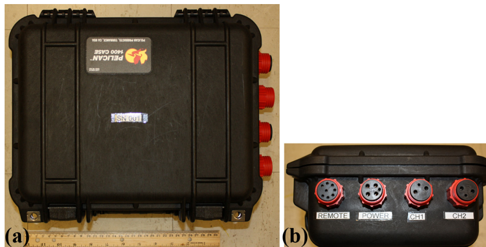
Figure 4. Non-submersible version of the Underwater Sound Recorder. (a) Pelican 1400 case; (b) external waterproof connections.
