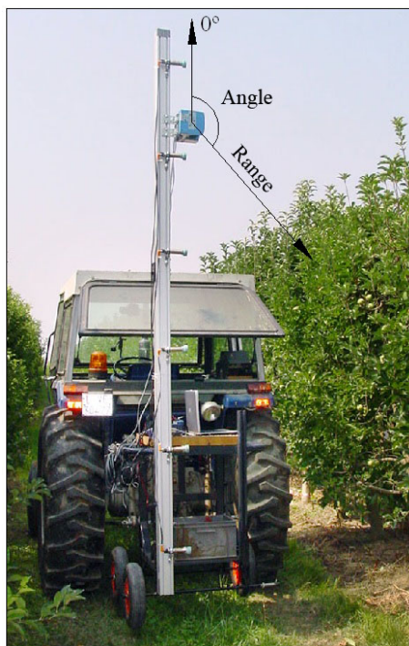
Figure 1. The impact points of the laser beam are determined by polar coordinates: range and angle.
