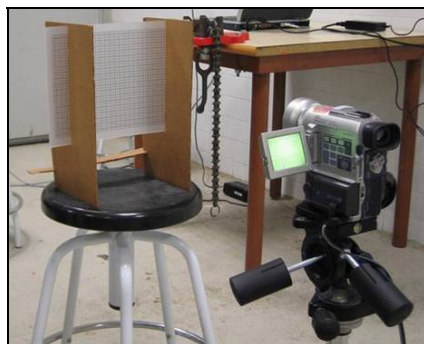
Figure 3. Plastic translucent grid template and digital camera used in characterisation of the laser beam.
