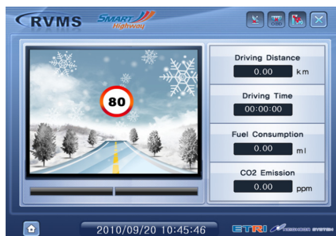
Figure 11. Example of a Telematics device with advisory speed and ice surface information.
