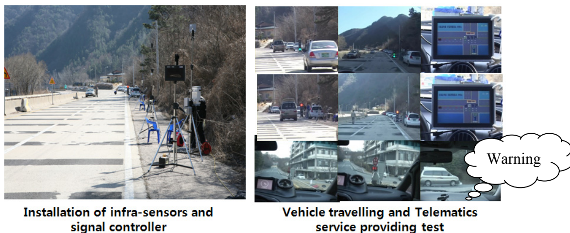
Figure 7. Signalized intersection test: red-light violation warning at signalized intersection.
