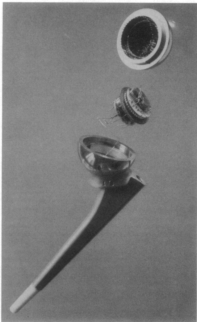
FIG. 1. Instrumented prosthesis showing pressure-instrumented pseudofemoral head hemisphere, electronics package, and antenna on distal end of intermedullary stem.
