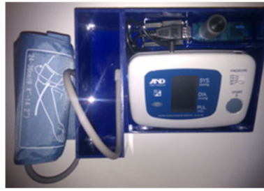
Fig. 5. Designed Bluetooth-enabled blood pressure monitor
