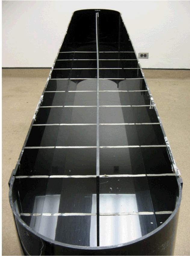
Fig. 1. The overhead view of the MDTB apparatus. The two 2-m straight segments of the oval runway are joined by two 0.4-m curved segments and separated by a median wall. The apparatus was elevated 0.8 m.
