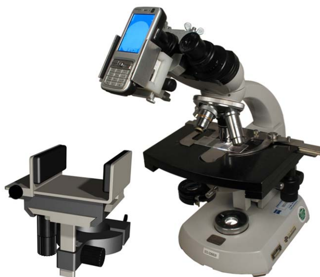
Figure 1. The prototype connector which attaches a mobile phone to a microscope. The prototype connector was designed by TU Delft and TNO. The connector is adjustable to fit all sizes of candy bar phones and some slide phones. It also consists of adjustable screws to fit most regular light microscopes. doi:10.1371/journal.pone.0028348.g001
