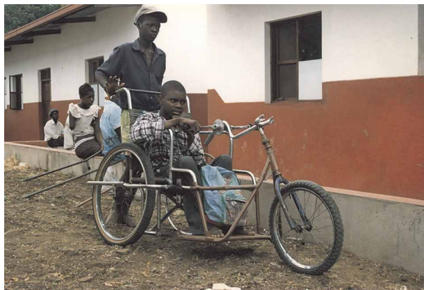
Figure 1 Hand-cycle wheelchair in Mozambique. A young man with paraplegia had to stop attending school after the chain in the arm cycle broke, and replacement parts were unavailable.
