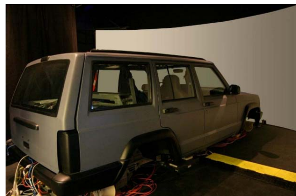
Figure 1 - The NADS-2 driving simulator with a Jeep Cherokee cab.
