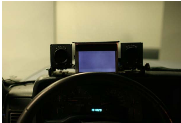
Figure 2 - The NVES display that shows simulated infrared image and visual warnings. Mounted around it are the eye-tracking cameras.
