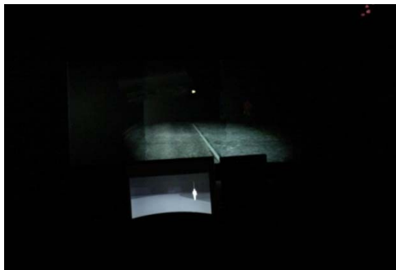
Figure 3 - Driver's forward out-of-windshield view and NVES display during a night time drive.
