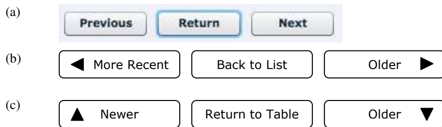
Figure 5. (a) Current buttons used to navigate between lab reports. (b), (c) Recommended button labels.
