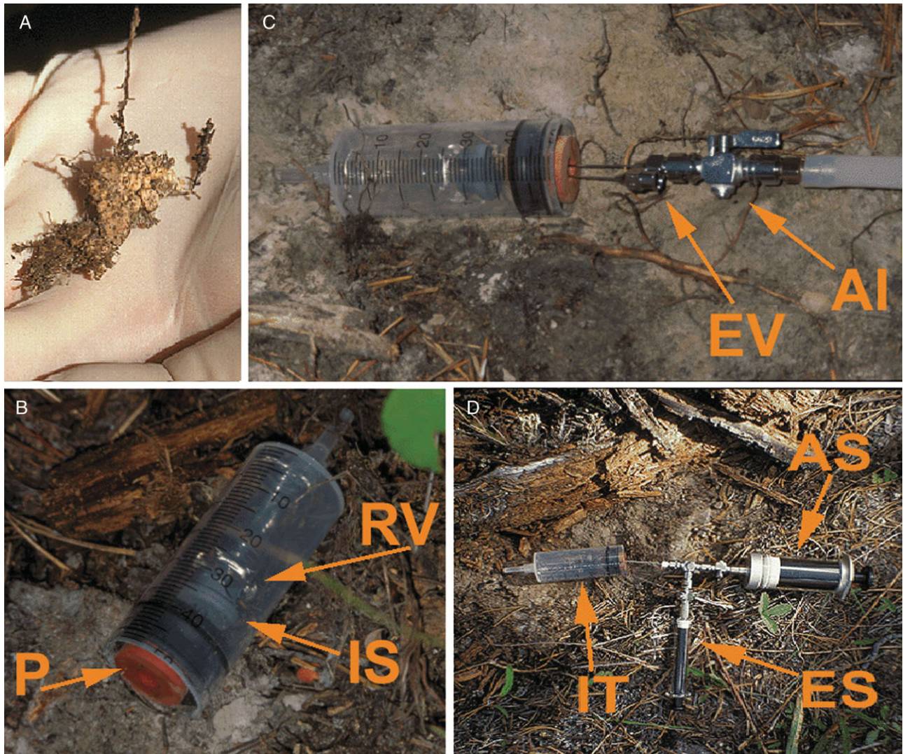
FIG. 1. (A) Pinus contorta root with Suillus tomentosus tuberculate ectomycorrhizae cleaned of woody material ready for insertion into incubation tube. (B) Acetylene reduction assay incubation tube showing plunger assembly (P) inserted, gas retention vial (RV) within incubation tube, and retention vial septum (IS) placed in the vial opening. (C) Acetylene reduction assay incubation tube being flushed with inert argon gas via the injection line (AI) and being vented by the evacuation needle (EV). (D) Acetylene reduction assay incubation system showing evacuation syringe (ES), argon injection syringe (AS) and incubation tube (IT).
