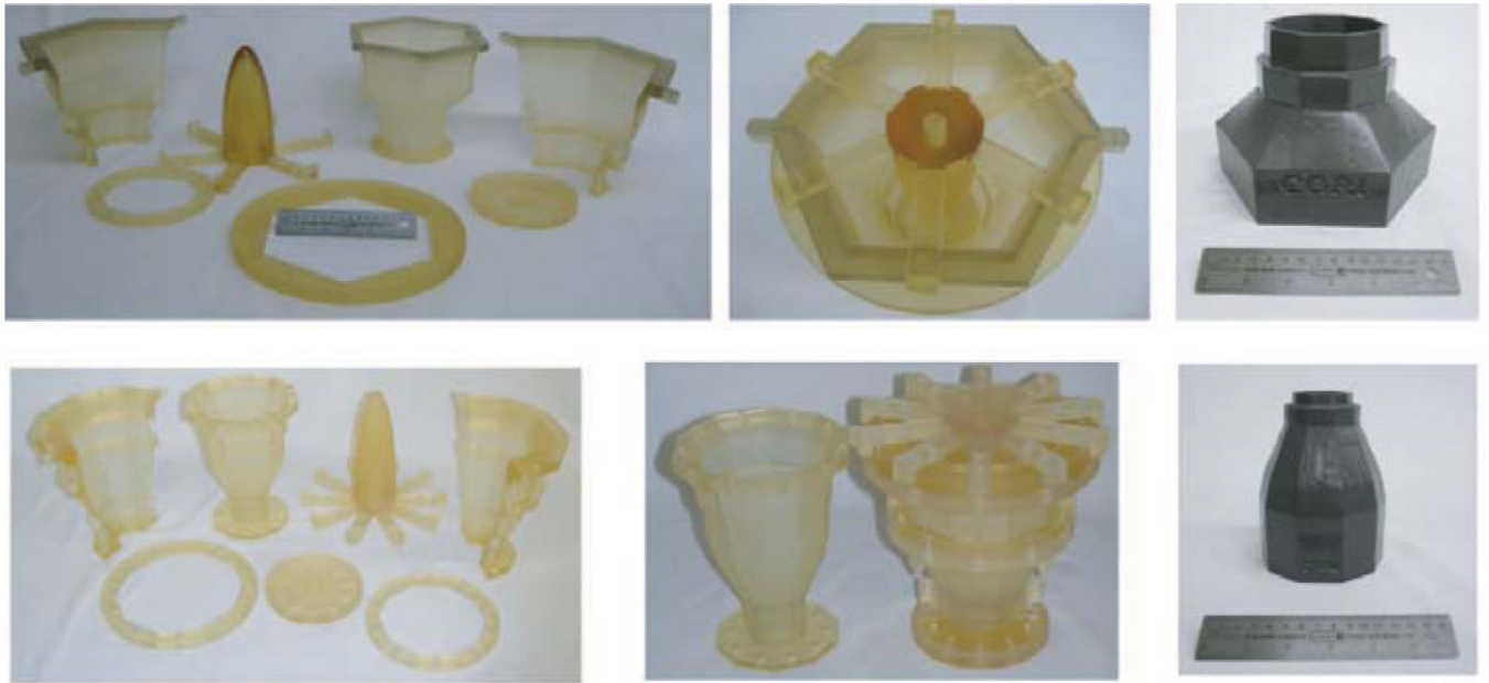
Figure 8. Mold assemblies printed on an Objet Connex350™ printer and the associated tungsten-composite cast pieces.
