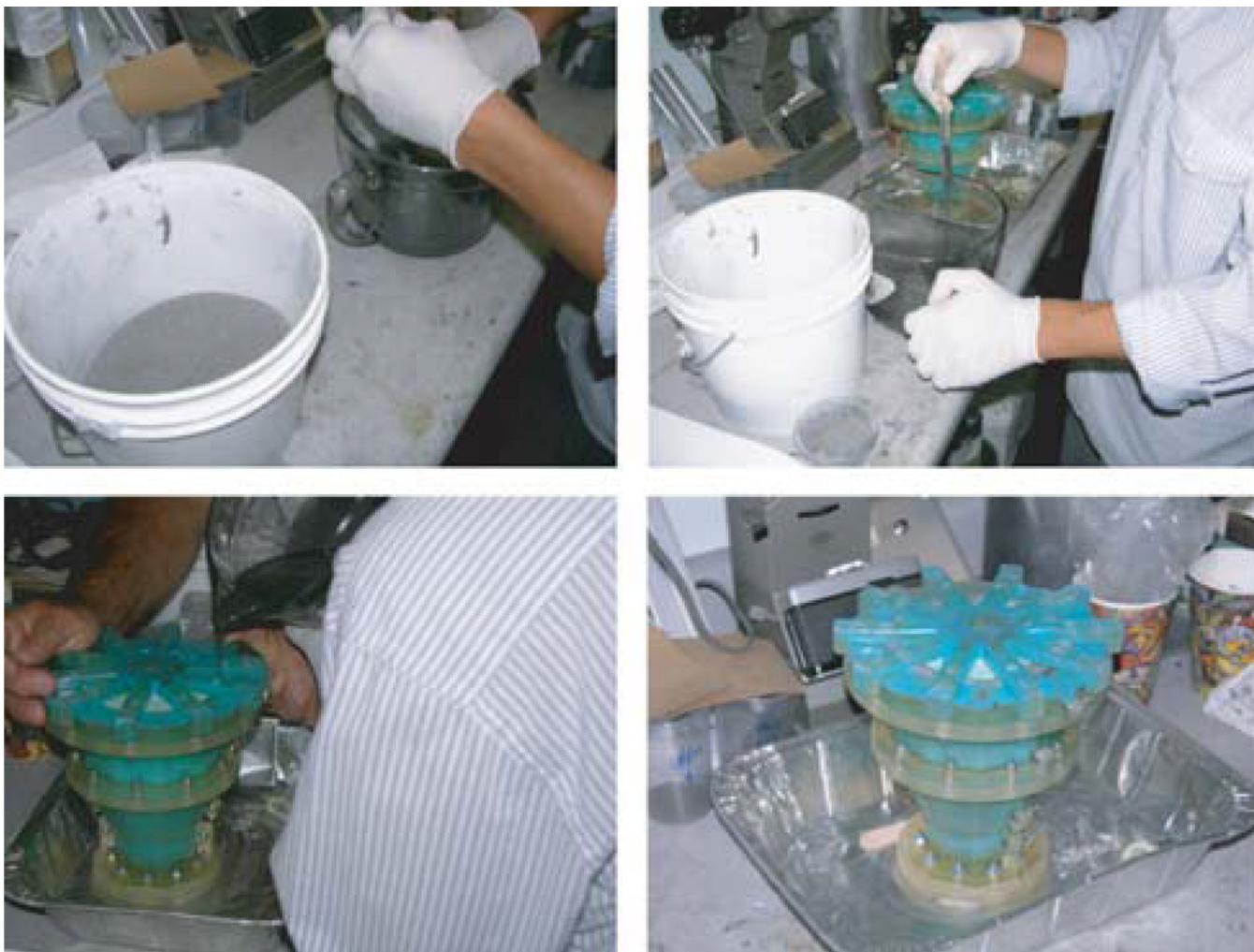
Figure 4. Tungsten Heavy Powder, Inc.[10] cold-casting process for creating high-density tungsten composite parts: a high-density tungsten powder is mixed with an epoxy and poured into a mold. The tungsten powder displaces the epoxy and settles to the bottom of the mold. After curing, the part is removed from the mold assembly and has a density \sim 9 \text{ g/cm}^3 .
