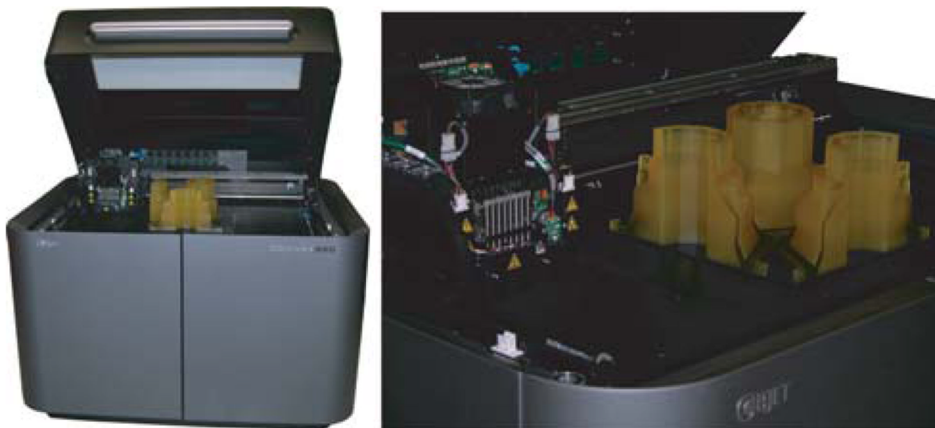
Figure 1. Objet Geometries Ltd.[8] Connex350™ printer. The tray contains printed parts for a mold assembly. The printer has a 35 \times 35 \times 20 \text{ cm}^3 build volume and prints slices 16 microns thick with a lateral resolution of 42 microns. Additionally, the printer is capable of printing in multiple materials to create parts having variable color, hardness, and flexibility.
