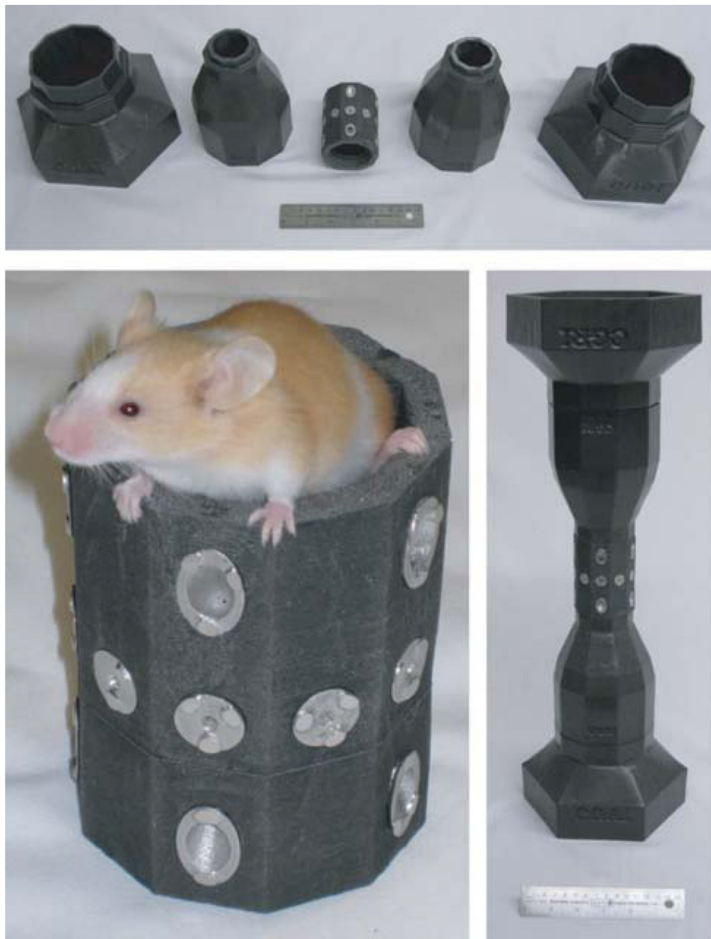
Figure 11. Complete FastSPECT III aperture assembly with platinum pinhole inserts and tungsten-composite supporting structure.
