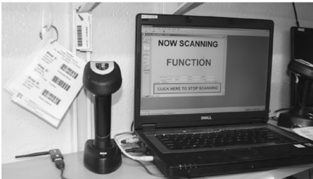
FIG. 1. The Aquatics Facility FileMaker Pro (FMP) database allows for easy and accurate barcode scan entry. (A) Actions, such as reporting that a tank of fish has been used for in vitro fertilization, can easily be entered by barcode scan. This demonstration illustrates the use of a handheld scanner, the scan guide, and the tank label. Also shown is the tank location label (on the rack). (B) Each station is composed of a laptop and handheld Bluetooth scanner, paired by serial number. This pairing allows for multiple stations and database users in one room.
