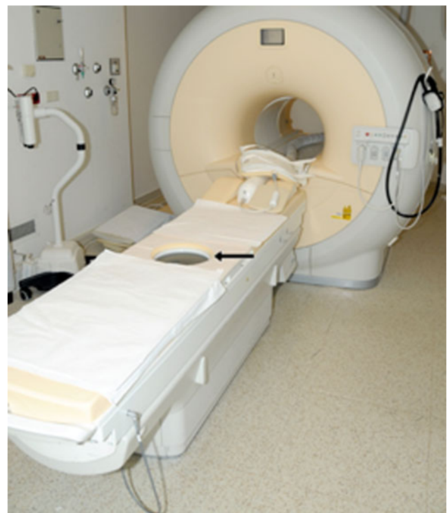
Fig. 1 The Sonalleve MR-HIFU system consists of a 1.5 T clinical MRI scanner and a 256-element focused ultrasound transducer integrated in the treatment table top
